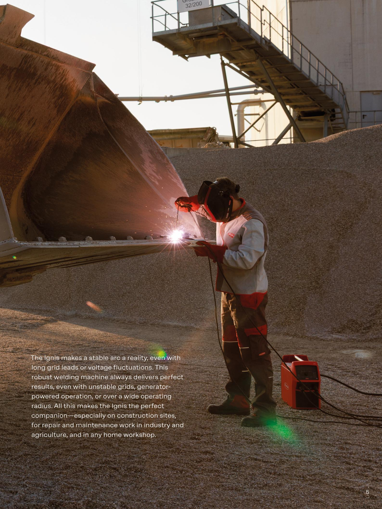
The Ignis makes a stable arc a reality, even with long grid leads or voltage fluctuations. This robust welding machine always delivers perfect results, even with unstable grids, generator-powered operation, or over a wide operating radius. All this makes the Ignis the perfect companion—especially on construction sites, for repair and maintenance work in industry and agriculture, and in any home workshop.
