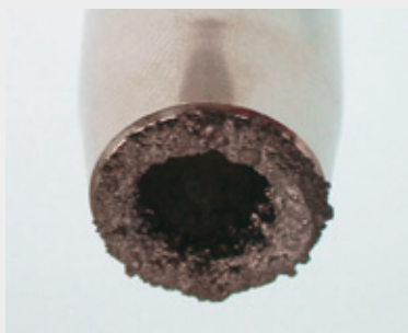
/ Gas nozzle with spatter build-up.
