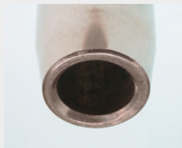
/ Gas nozzle after touchless cleaning.
