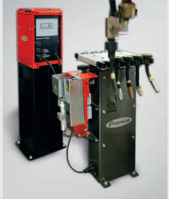
*/ With Robacta TX, the welding cell becomes increasingly autonomous. The change of torch-body takes place within 30 seconds, without human intervention and independently of work-shifts. Robacta TX is available for water- and gas-cooled welding systems with pay-off packs.*
