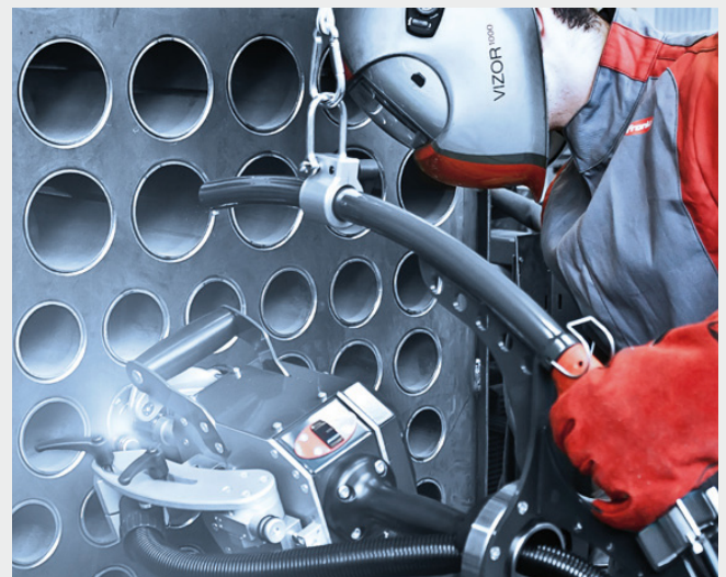
/ Horizontal welding position
